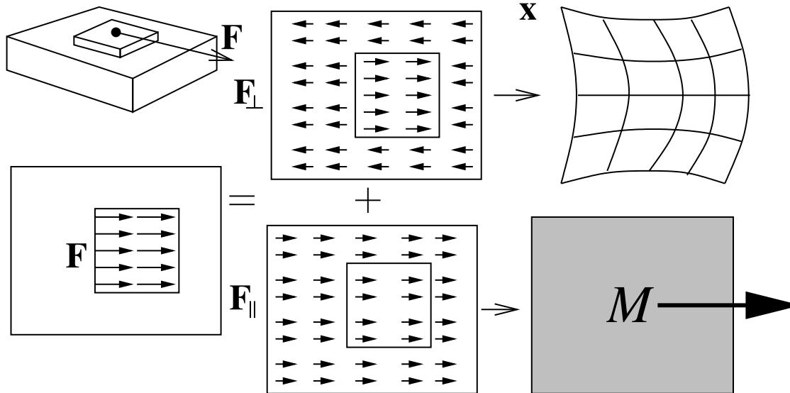
Only a limited number of functions are needed to describe the internal motion for a given applied force. However, for every fixture independently
